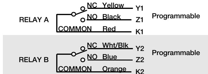
Figure 4. 2-relay output color coding
