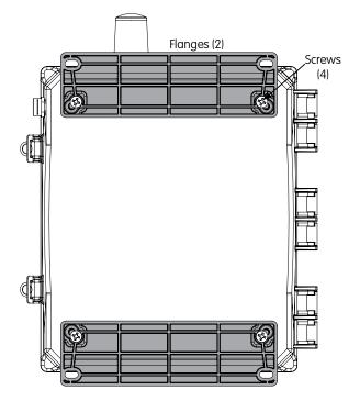
2. Position the pole mounting bracket so that the orientation matches the following illustration. Be sure that the ground lug is in the correct position.
