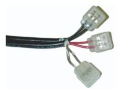
6. Provide strain-relief by securing the two cables together using the cable ties.
