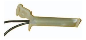
9. Close the insulator tube. Be sure that the cables exit the tube from opposite sides.
