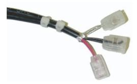
7. Arrange the gel splices along the cables in a single column. Be sure that the bare wire splice is aligned down the cable (left-most splice in the following illustration). Because the bare wires are not insulated, they are not as rigid as the others. With the bare wire splice facing down, it will be easier to insert into the insulator tube.
