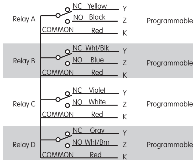
Figure 6. Relay output wiring for 4 relays, 9 wires
